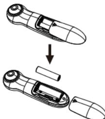
3. Reinstall the battery cover as shown by the graphic to the right.
